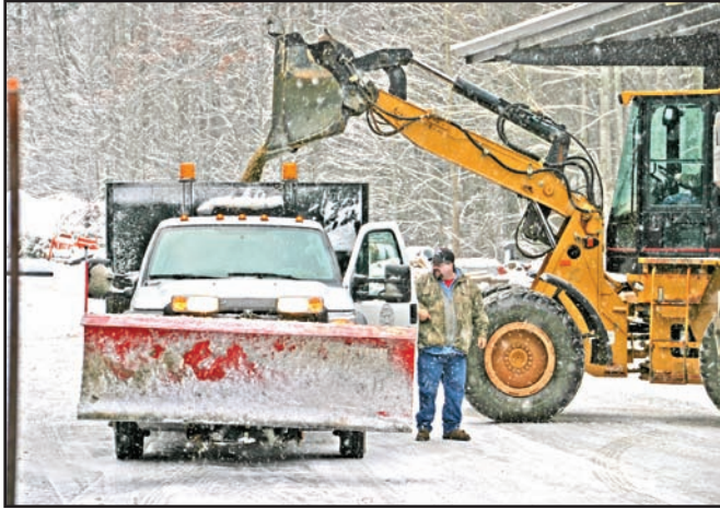
David Land with the Union County Road Department stops in to headquarters early Saturday morning to refill his truck with the salt/gravel mixture used to treat icy roads
